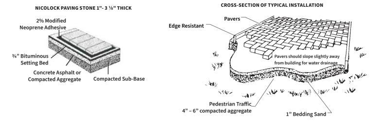
NOTE: All measurements are nominal. Variance in square footage or linear footage coverage can be up to 5% depending on joint width. The possible occurrence of efflorescence does not affect the structural integrity of the product. Efflorescence is a normal occurrence in concrete products and will dissipate with normal weathering. The use of concrete as a base or setting bed may increase the possibility of efflorescence.
